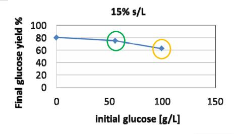
Glucose was slightly inhibiting toward the hydrolysis of fresh biomass at 15% s/L and enzyme-to-glucose ratio of 0.15 g/g.
