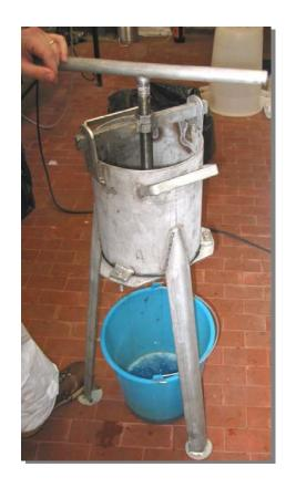
After the pretreatment the solids were separated from the liquid and then recombined up to the desired DM level
