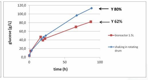
In vertical bioreactor, the addition of fresh biomass at 72 hours did not increase the glucose yield
